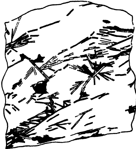
FIG. 186.—Section of ore from Chestnut Yard, Va., showing pyrrhotite (white) and chalcopyrite (black) replacements in hornblende (parallel lines). (After Weed and Watson, Econ. Geol. , I.)
